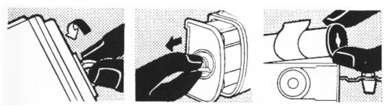
Unloading. Wind off the end of the backing paper with the loading key (left), then remove the spool holder by unlocking the spool key and withdrawing the holder (centre). Finally remove the full film spool and seal (right).
