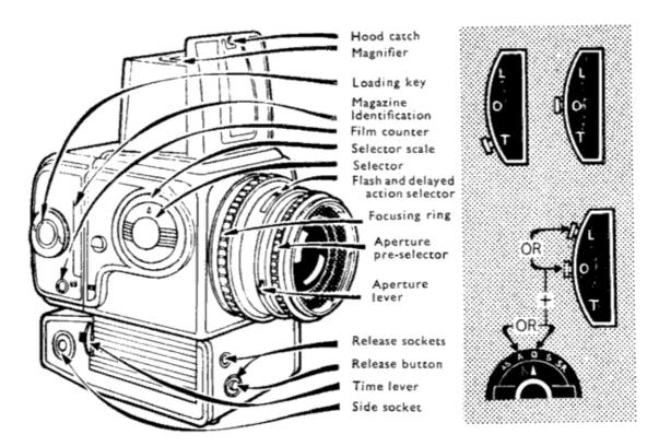
The 500EL is basically a 500C, but it has additional controls. The time fever, shown at right above, is used for exposures from 1 second to 1 minute and when making exposures with the self-timer. Moving the lever to T (with the shutter set to B) opens the shutter. Moving the lever to O closes the shutter, advances the film and recocks the shutter. When changing lenses, the time lever must be set to L or O and the selector scale (see below) set to A or O.
