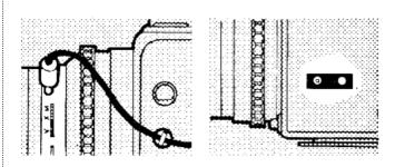
The flash cable plugs into the socket lever (left). A cable bearer fits into one of the two sockets in the left hand side of the camera to prevent accidental pulling out of the cable.
