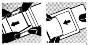
To load the cut film holder place the trimmed sheet of film below the film frame (left), fold down the latter and push in the sheath (right). This must be done in total darkness.
