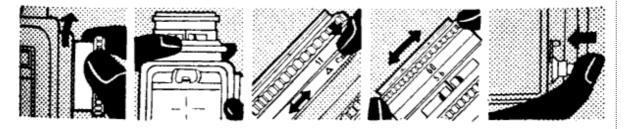
Shooting with the 500C. From left to right: Wind the film transport; view and focus the image on the screen; set the exposure value; select a suitable aperture-speed combination; press the release to expose.
