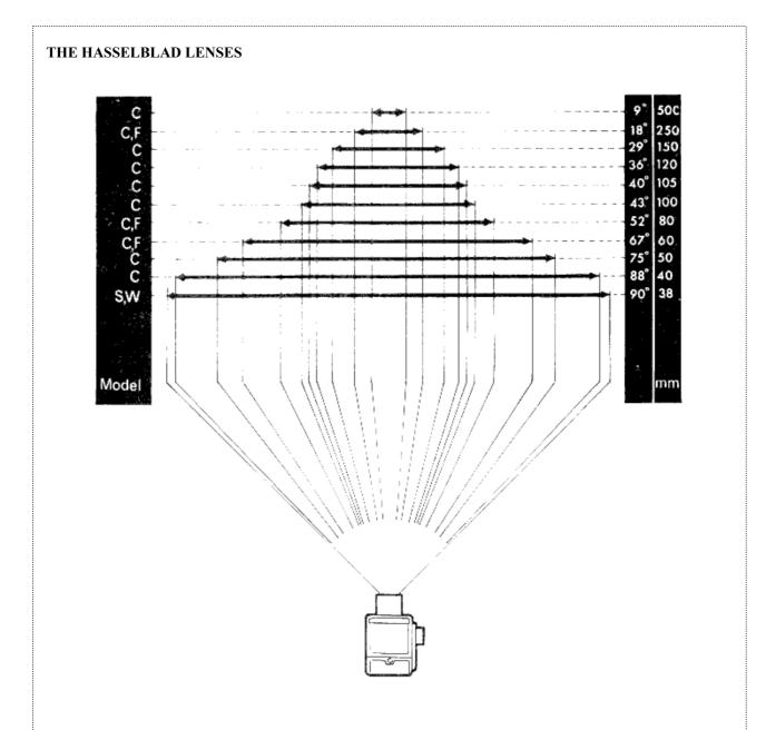
The shorter the focal length of the lens, the greater the angle of view taken in. With the interchangable lenses the Hasselblad can thus control the angle of view - and also the scale of the image recorded.
