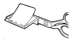
The film cutter cuts down  $2\frac{1}{2}$  x  $3\frac{1}{2}$  in. sheet films to  $2\frac{1}{2}$  x  $2\frac{1}{2}$  in. To trim the film, push it under the cover guard so it touches the stop pins. Then trim the film with the built-in scissor blades. This also must be done in total darkness.
