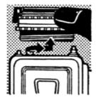
To remove the lens on the F models press the catch (left) and turn the lens anticlockwise to lift out (right).
