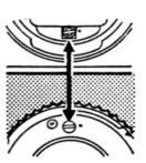
To fit the lens, mount on the camera so that the red marks on the lens and body are in line (left), then turn the lens clockwise (centre). The tensioning shafts on both the camera and the lens must have their groove lined up with the red dot before a lens can be fitted (right). This is automatically the case if the camera is always tensioned before a lens is removed or fitted.
