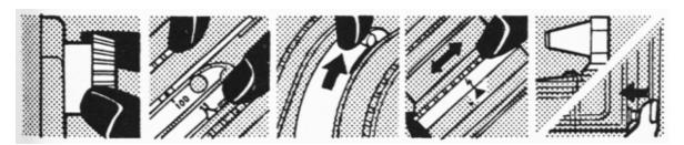
Shooting with the Super Wide. From left to right: Wind the film transport knob; set the aperture and shutter speed separately; tension the shutter; set the lens to the appropriate subject distance; view the subject through the finder and release the shutter.
