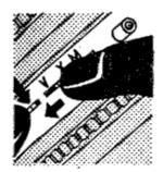
Left: To use the self-timer set the synchronizing lever to the position V, while pressing the locking catch next to it. This must be done after tensioning the shutter. The time catch must also be set to T. On pressing the release the shutter opens after a delay of about 8 seconds.
