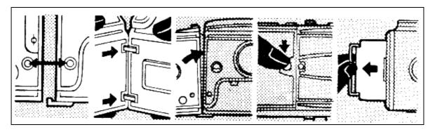
Fitting the magazine. Check that the signal on the camera and magazine correspond (left), then hook the bottom of the magazine to the camera body (centre left), push the magazine against the camera back (centre), and secure the catch (centre right). Then pull out the slide (right); the camera is now ready to shoot.
