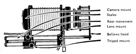
The extension bellows can also be used for copying transparencies with the aid of the transparency copy holder. This fits on the front of the extension hood and takes transparencies (or negatives) which are illuminated from behind by suitable light source.
